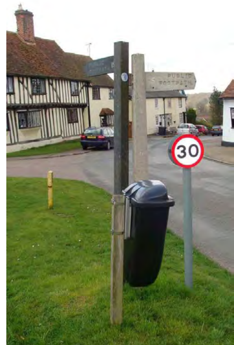
Picture 1.24 Uncoordinated street furniture on the central green west of the church yard. Cannot the opportunity be taken to simplify this arrangement where 2 no footpath signs, a litter bin and a 30 mph sign each have separate post supports?
